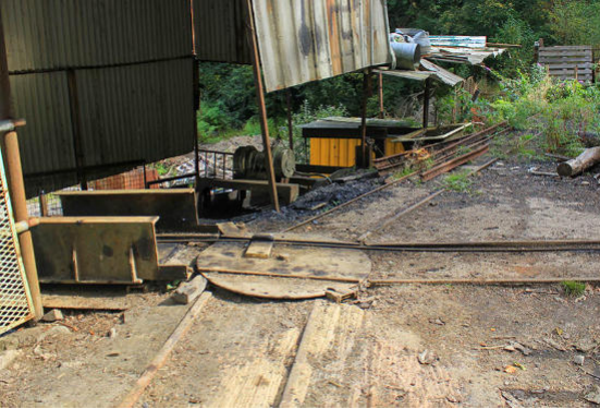
Above left: Monument Mine – railway layout for access to sieving; note the use of a wagon turntable Above right: General view of the Reddings Level Mine. The mine access is in the rock face to the right of the blue barrel. Mined coal is taken to the upper level on the left near the blue compressor for sieving Below Wallsend Colliery (left) The entrance to the mine, and (bottom right) the steep route of the railway from the mine entry/exit. The sieving equipment is beyond the blue tarpaulin on the left
